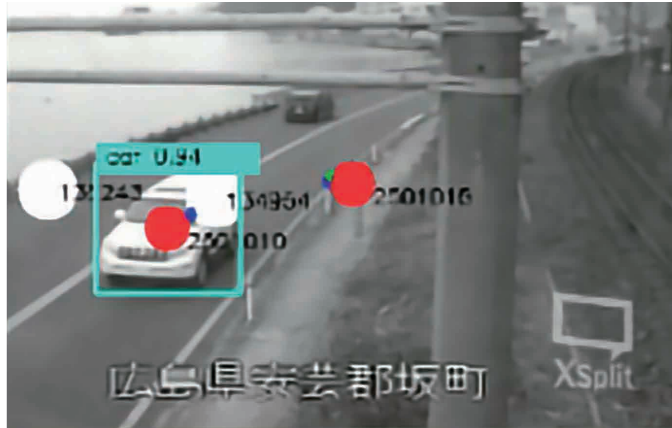
Measuring traffic volume by AI analysis of CCTV feed (e.g., During heavy rain in July 2018)
