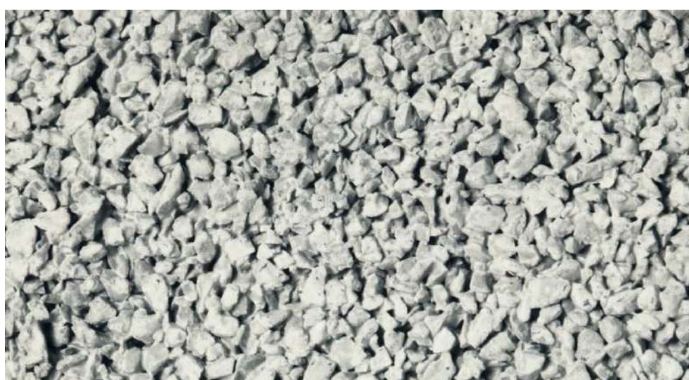
▲ Medium grain aggregate grain diameter 2.5 to 5 mm
