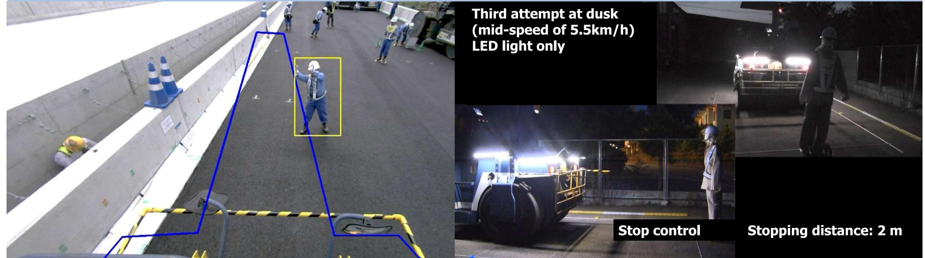
The advanced image analysis system will detect human presence even when only a person's foot gets inside the defined detection area. The yellow frame shown above indicates that the system has recognized human presence in the control distance range so that the vehicle will be automatically slowed down by the control unit.
