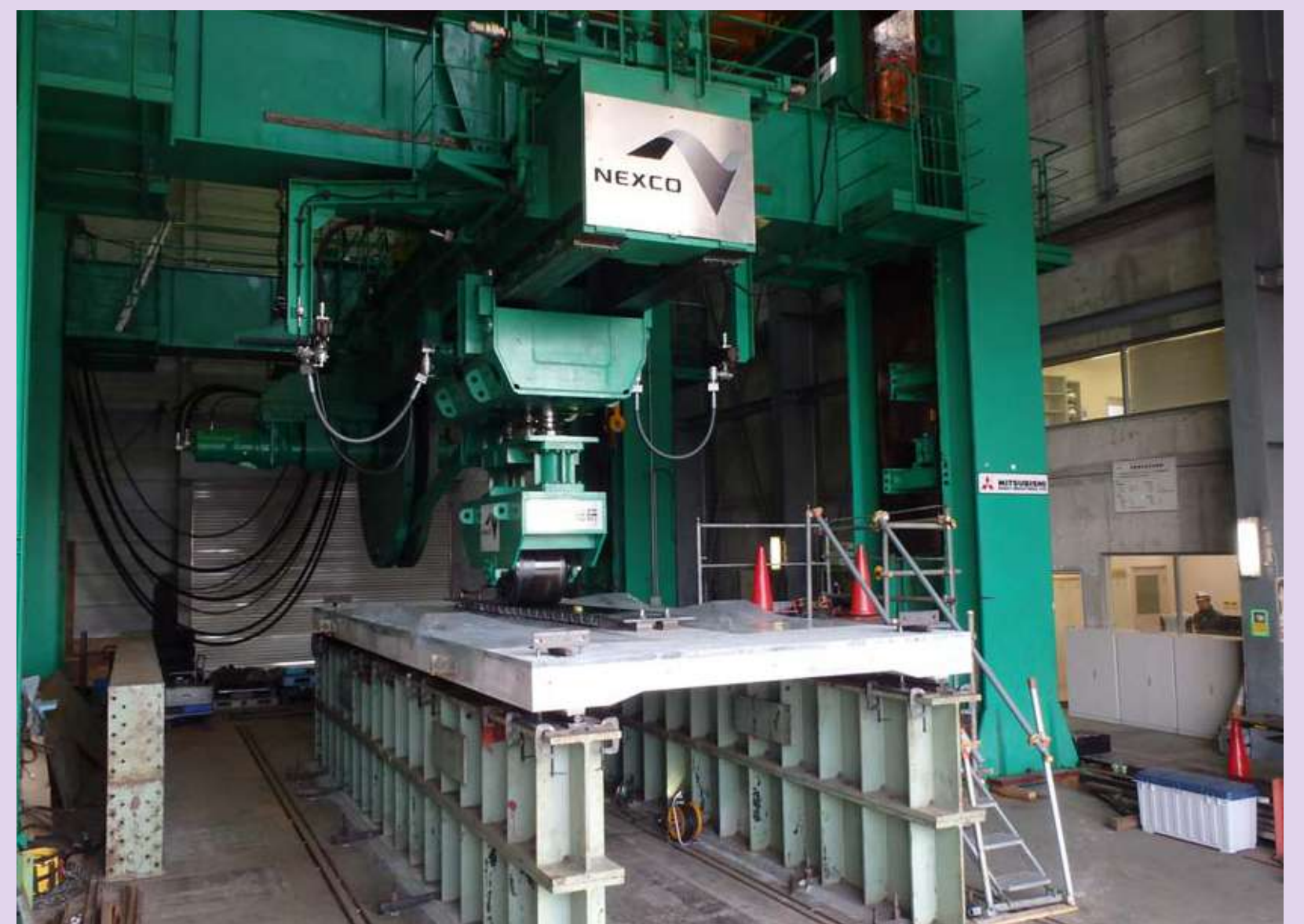
Dynamic wheel loading test
