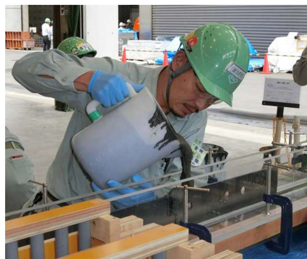
Gap filling test with fluidity-enhanced UHPFRC
